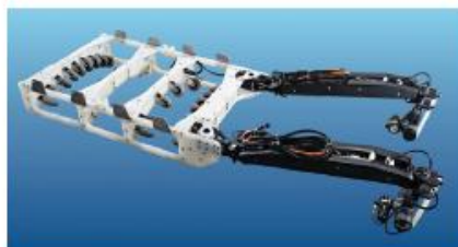
PIPELINE SURVEY WHEELED SKID WITH BOOM ARMS
